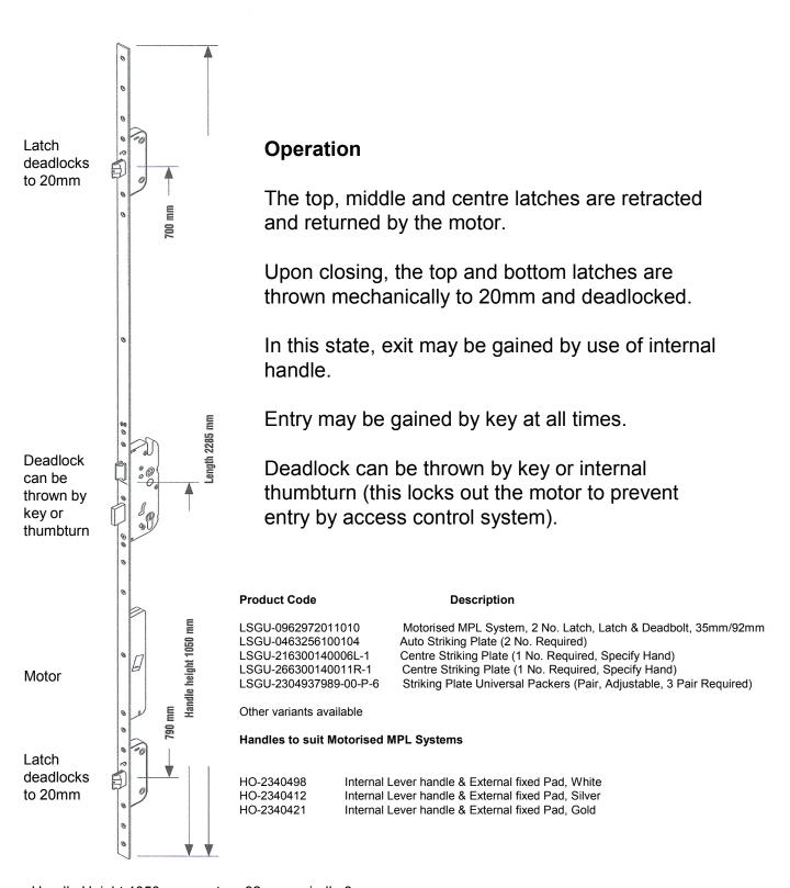
Handle Height 1050mm, centres 92mm, spindle 8mm
